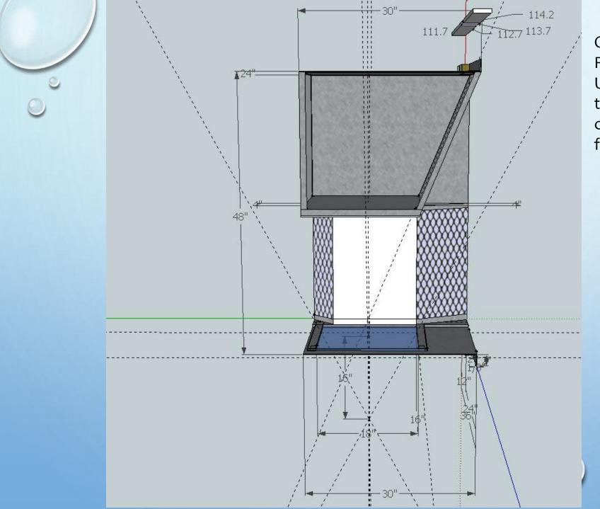
Over head view Flow from left to right Unit slides into current trash rack bracket and is completely external of fishway
